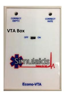
The VTA box with light indicators runs on a 9V DC battery installed in the back of the VTA box. To turn it on, slide the switch to the on position. The lights that indicate correct depth and correct rate will blink while the VTA box is orienting and calibrating. Compressions can begin once the lights stop blinking.
